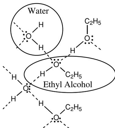
**Figure 1.** Hydrogen bonding between alcohol and water.
