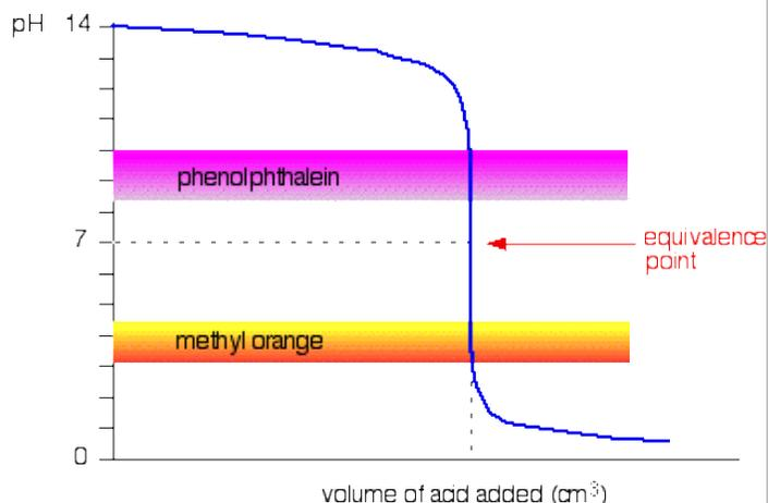
pH indicator phenolphthalein is used because it changes colours near the equivalence point
